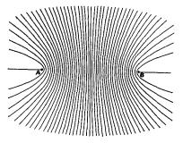
The nature of the lines of position when stations are many wavelengths apart. Note the uniform spacing along the baseline, the gradual increase in spacing transverse to the baseline and the marked increase in spacing behind the transmitters (A and B).
