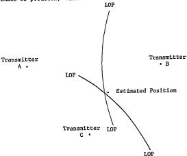
However, the diagram over-simplifies the situation. A position-fix is obtained, not by drawing intersecting lines on a map, but by drawing intersecting bands, with each band making some allowance for errors and deviations from a theoretical centre line. The result is a quadrilateral where the bands intersect, not a point. A navigator can then construct a circle, its centre at the centre of, and its radius derived from, the
